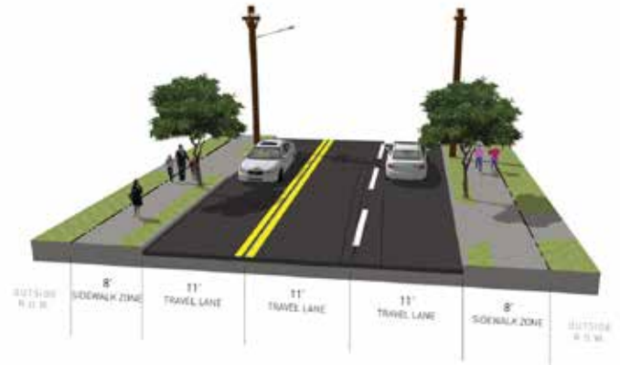
MONROE DRIVE: EXISTING TYPICAL CONDITION
