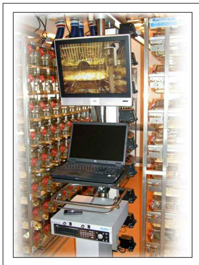
Figure 3: Rack-mounted closed circuit video cameras permit remote monitoring of animal activities within cages.
